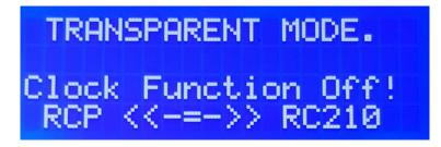
The above display will confirm the clock has moved to Transparent Mode. Although the clock is still receiving G.P.S. Information no updates are passed to the RC210 repeater controller. To exit this mode simply press [ENTER], The G.P.S.CLOCK will immediately update the RC210 with current G.P.S. Time.
