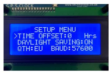
The Cursor changes to a  $\rightarrow$ . At this point the **UP** and **DOWN** buttons change the value show. Press **ENTER** to set the value.
