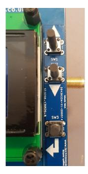
To the right hand side of the main display are located 3 push buttons. From top to bottom these are [UP], [DOWN] and [ENTER].
